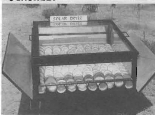
Modified Solar dryer Using selectively coated aluminium absorber sheet.
